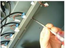
Remove the broken ink pump and remove the tubes connected to the pump. Illustrated as below.
