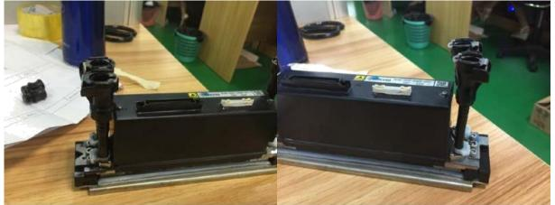
Finish the connecting between sub tank to heads and fix the printhead
