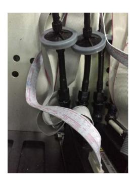
Finish installing the printheads one by one
