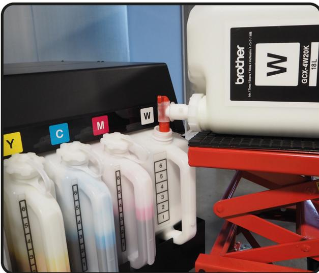
This tool will help you to **move the bulk ink tanks** from the boxes to the printer and **to fill-in** the tanks clean and easy.
