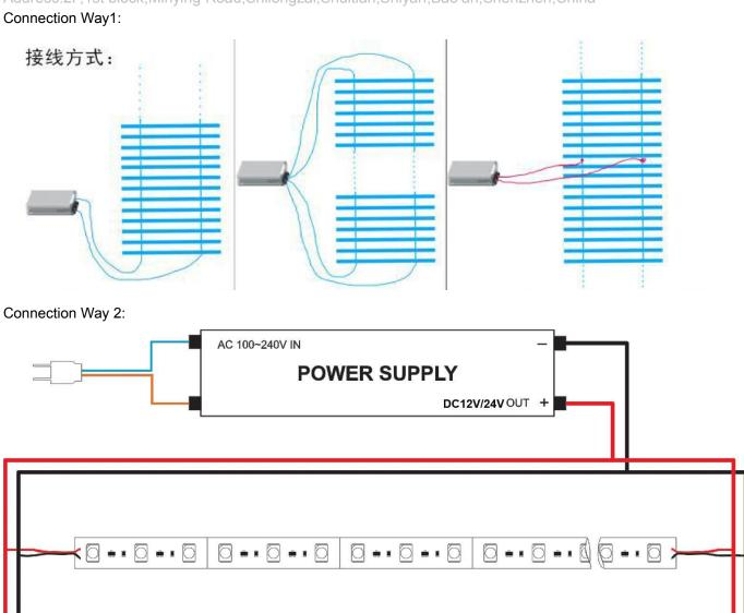
parallel connection and also connect the both ends of led strip lights to the power supply
